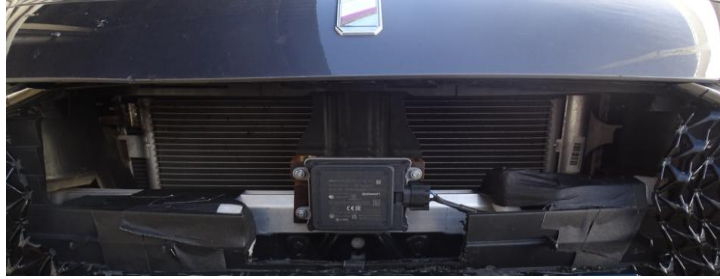
Figure 2. Radar sensor installed in the VUT front grill
