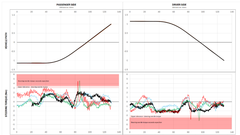
Figure 17: Observation of steering torque requirement - 0.6m/s – Solid line marking
