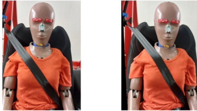
Figure 1: Comparison of belt positions in pilot 1 between the one used in the tests (left) compared to the one where it was tried to match the position used in the simulations as close as possible (right)
