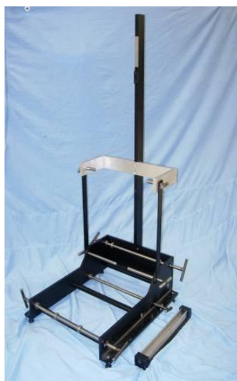
Figure 24: HPM Calibration Jig (GLORIA)
