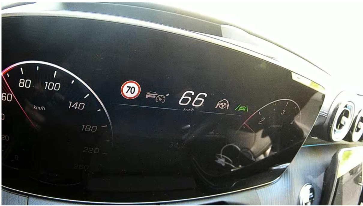
Figure 8. Desired quality of a dashboard image. Note that the SLIF icon and speedometer info are quite clear, with limited reflections.
