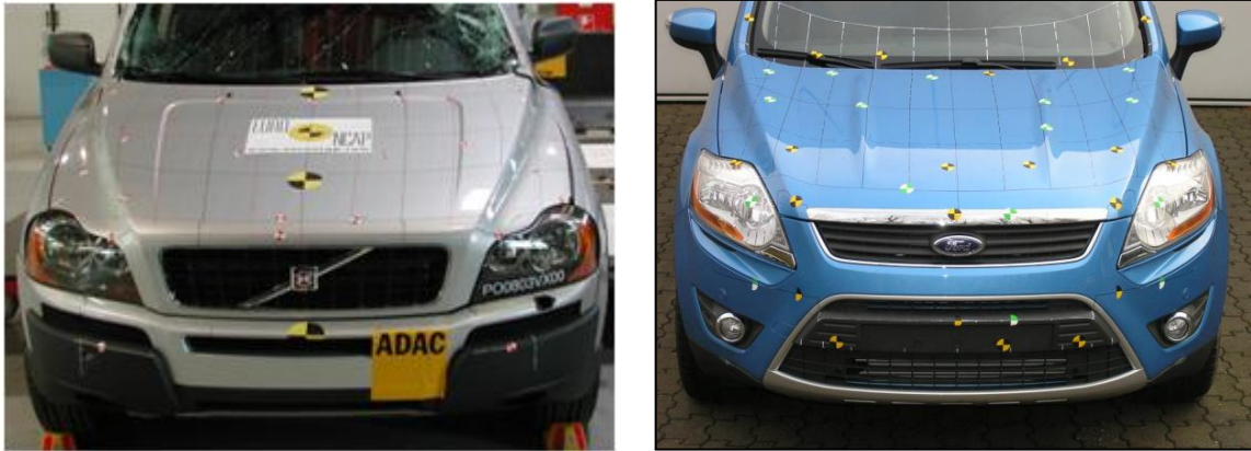
Examples of vehicles where the BLE located between WAD 1000 and WAD 930
