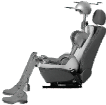
Figure 2. SAE J826 H-point manikin combined with Head Restraint Measuring Device (HRMD).
