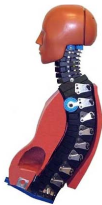
Figure 4. Cross-sectional view of the BioRID upper torso, showing its segmented spine for human-like response and seat interaction.
