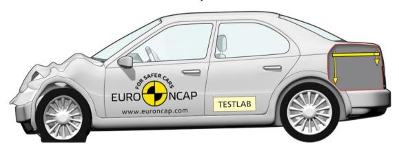
Figure 2. Re-setting axis reference frame after test.
