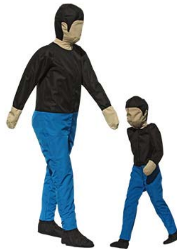
Figure 4. Euro NCAP Pedestrian Targets (EPTa & EPTc)
