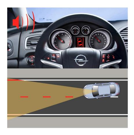
Opel Eye uses a camera at the top of the windscreen to monitor the area in front of the vehicle. Information from the camera is continuously analysed to identify road markings and traffic signs. Road markings are used as the basis of the first of Opel Eye's two functions: lane departure warning. Traffic signs are recognised and indicated to the driver in the second function: traffic sign memory. Euro NCAP has assessed and rewarded Opel Eye on the basis of its lane departure warning function.
