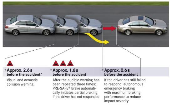
\*Time calculated by the system until the impact where the relative speed remains unchanged
