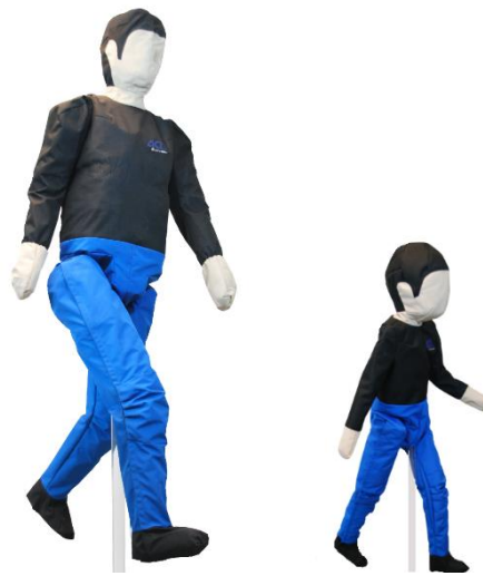
Figure 5: Euro NCAP Pedestrian Targets (EPTa and EPTc)
