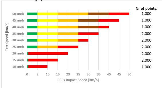
For each predicted colour the following scaling is applied to the grid point:
