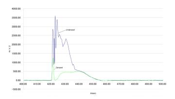
J-NCAP started using damped accelerometers for pedestrian testing in 2003. The issue was widely discussed during the development of the ECE global technical regulation (GTR) for pedestrian protection<sup>2</sup>. The GTR, published in 2007, requires the use of damped accelerometers for all child and adult headform tests.
