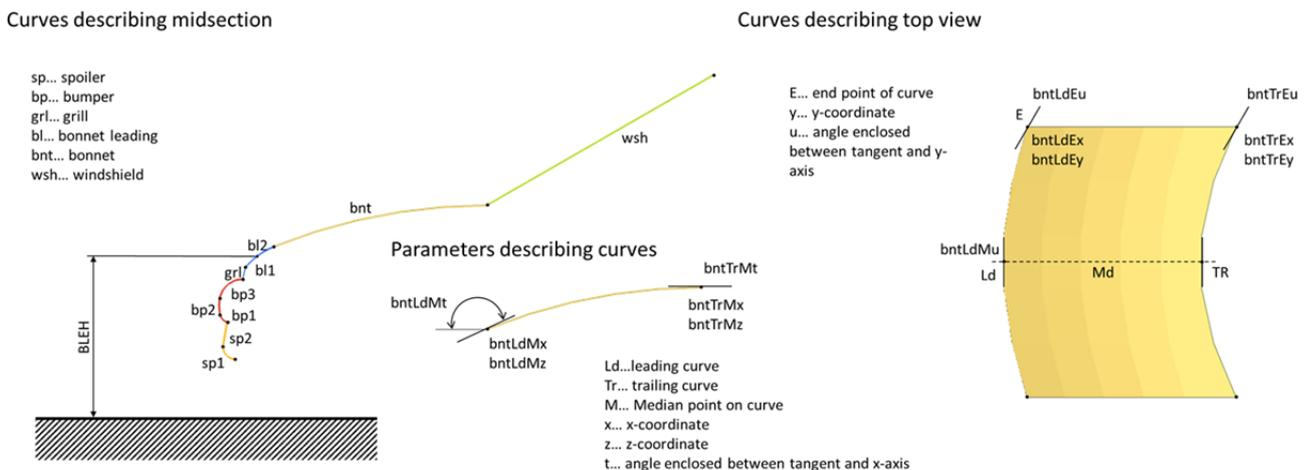
Fig. 1: Parameters of Bézier curves defining the vehicle geometry
