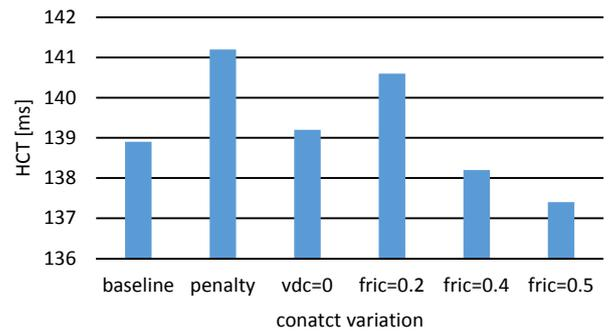
Fig. 21. Sensitivity of HCT to modifications of contact options (THUMS impact with generic family car model at 40 km/h).
