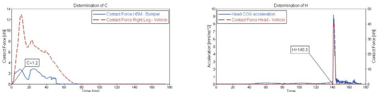
Fig. 3: Determination of Head Contact Time HCT= H-C.
