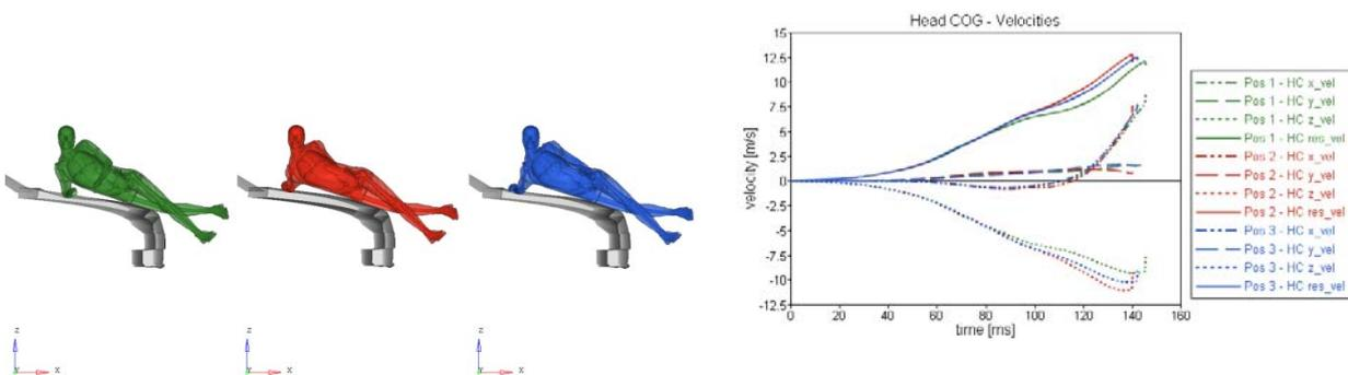
Fig 18.: Support of humerus for Posture 1 (left) and 3 (right) at 100 ms (FC with 40 km/h, GHBMC).
