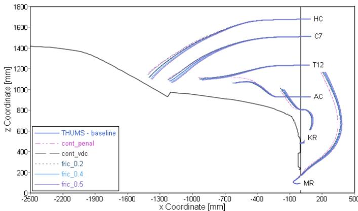
Fig. 20: Sensitivity of Trajectories to modifications of contact options with THUMS (impact with generic family car model at 40 km/h).
