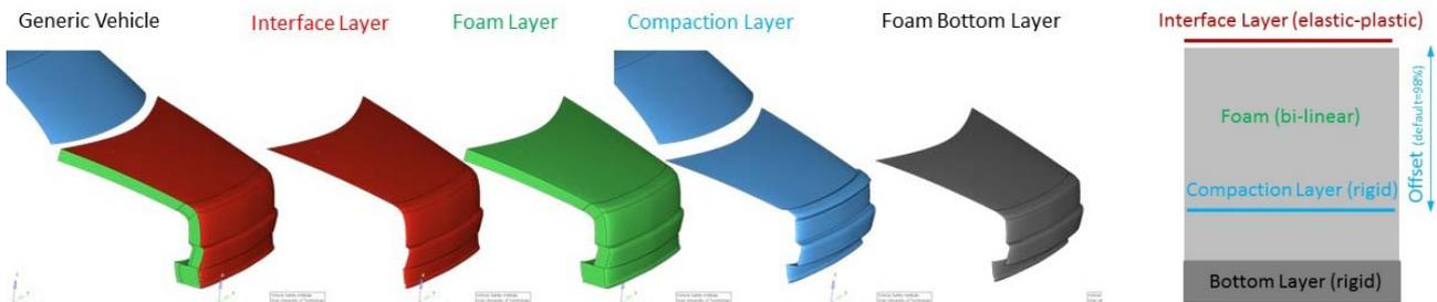
Fig. 2: Layers forming the GV models.
