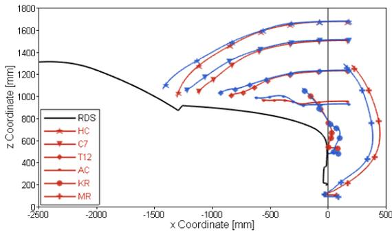
Fig. 22: Comparison of trajectories of THUMS (blue) and GHBM (red) for the impact with the generic roadster model at 30 km/h.
