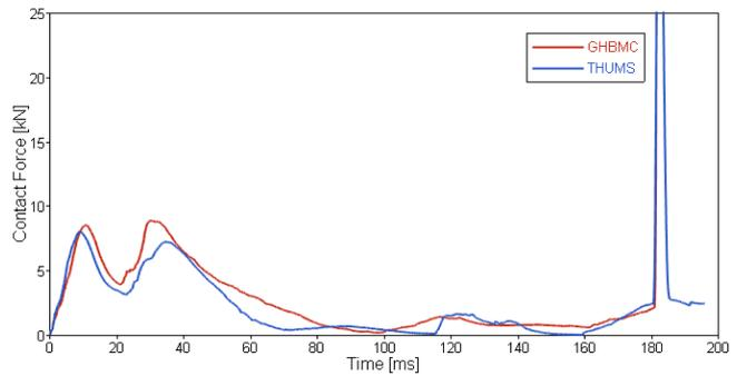
Fig. 23: Comparison of contact forces of THUMS and GHBM for the impact with the generic roadster model at 30 km/h.
