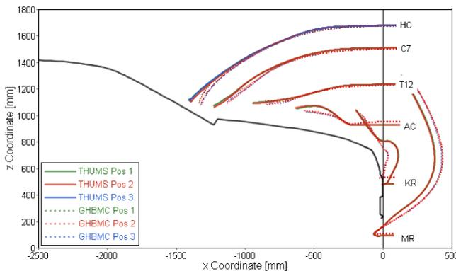
Fig. 16: Influence of initial arm posture on trajectories (impact with generic FC model at 40 km/h)
