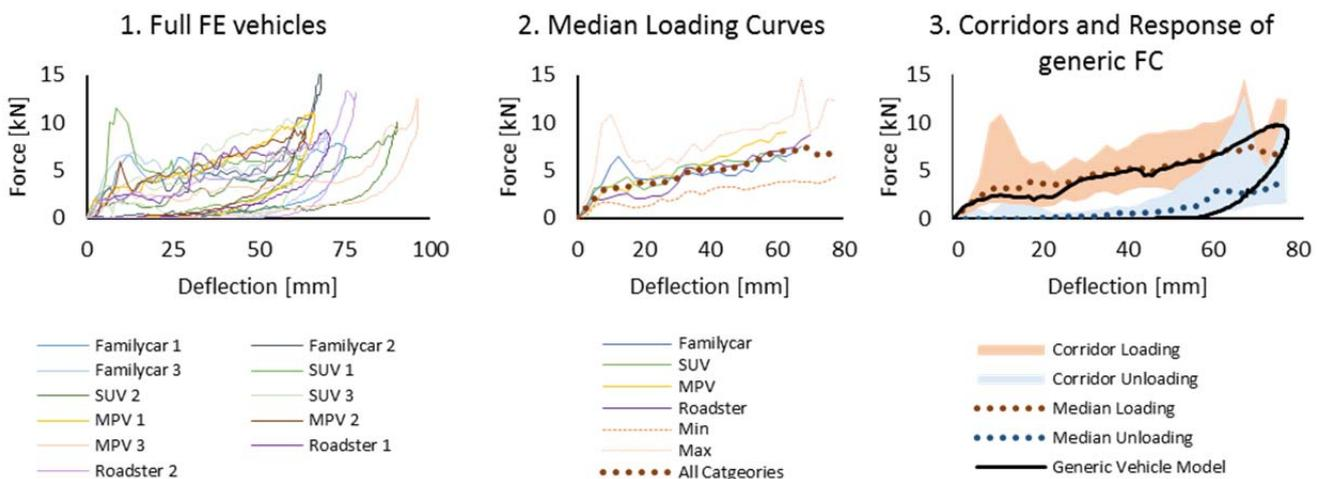
Fig. 7: Force deflection characteristic of single vehicles for impact simulations at bumper centreline.
