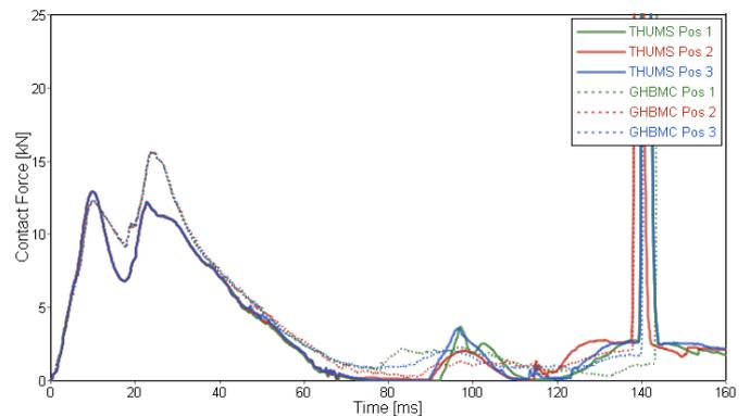
Fig. 17: Influence of initial arm posture on total contact forces. (impact with generic FC model at 40 km/h)
