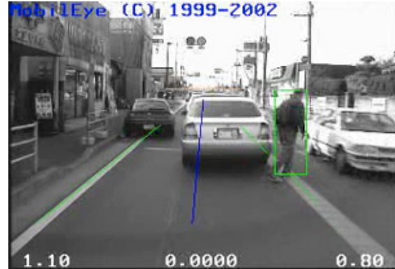
Figure 6 - Example of detecting a crossing pedestrian with a mono video system
