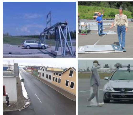
Figure 14 - Examples of test set-ups: Portal rig (top left), movable platform (top right) and cable pedestrian rigs with dummy suspended from cables (bottom right) and pulling cable running over surface (bottom left).
