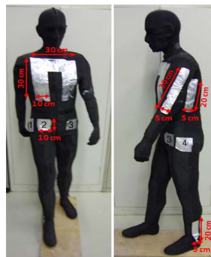
Figure 13 – Reflective foil used for scattering on one of the targets (spotty scattering centres)
