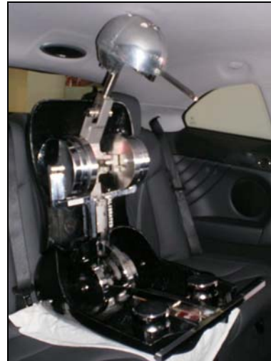
Figure 5. HRMD cannot be levelled, alternative measurement method required.
