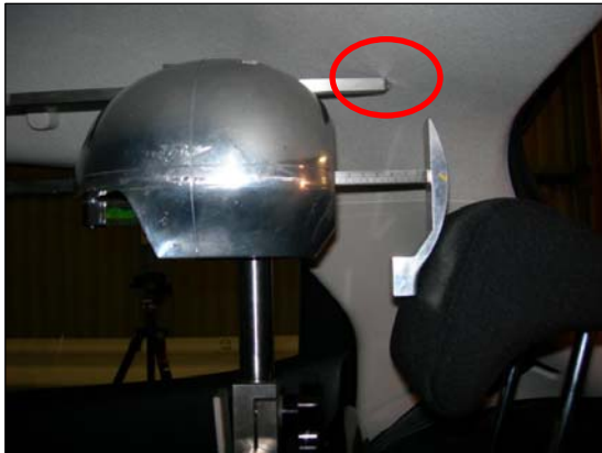
Figure 3. Height probe interference with roof lining.
