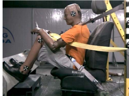
Figure 7-a : Test 2 – HII dummy position at 58ms – lab belt still on the pelvis
