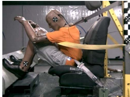
Figure 7-b : Test 2 – HII dummy position at 73ms – lab belt in the abdomen
