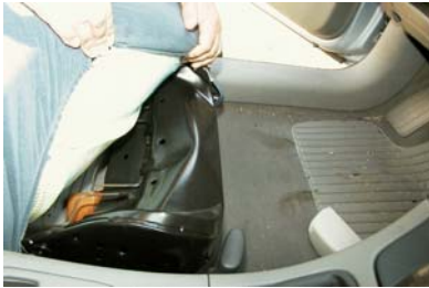
Figure 18 : front seat after real accident – pelvis impact on anti-submarining ramp
