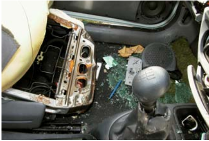
Figure 2 : collapse of the seatbase structure
