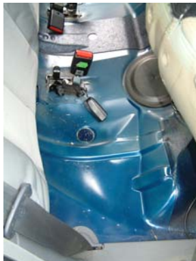
Figure 19 : rear seat after real accident – pelvis impact on anti-submarining ramp
