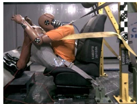
Figure 4 : Test 1 – HIII dummy position when maximum pelvis forward movement is reached
