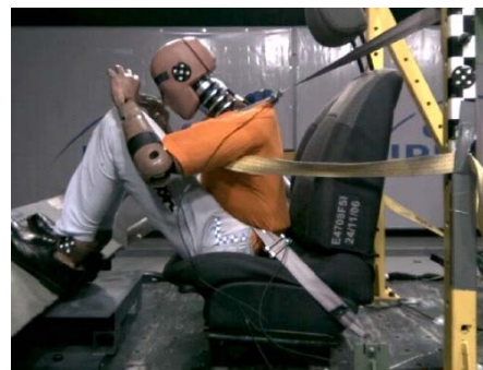
Figure 12 : Test 3 – HIII-FAA dummy position at 73ms – lab belt in the abdomen
