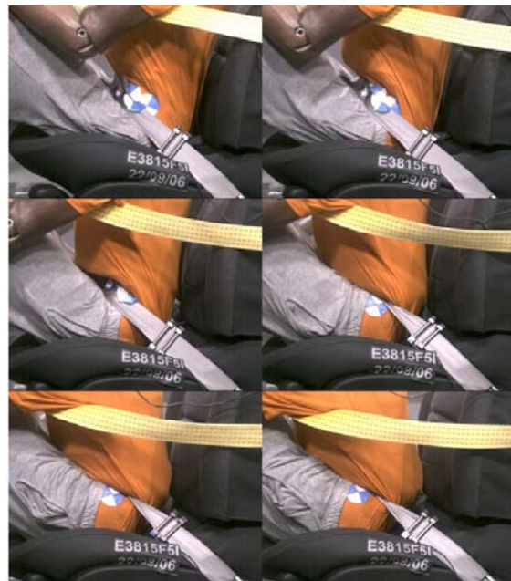
Figure 8 : Test 2 – HII dummy submarining sequence (from 50 to 75 ms)
