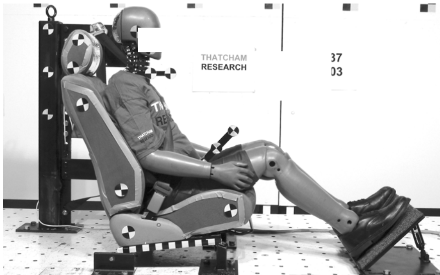
Figure 4. The BioRID II c placed in a Toyota Corolla seat on the Hyper G sled.
