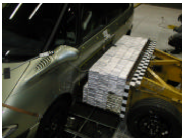
Figure 2: Side Impact test according to EuroNCAP.
