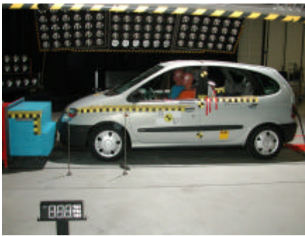
Figure 1: Frontal test according to EuroNCAP
