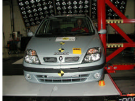
Figure 3 : Pole test according to EuroNCAP
