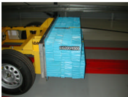
Figure 7 : The type of barrier used in the present EuroNCAP side impact test.
