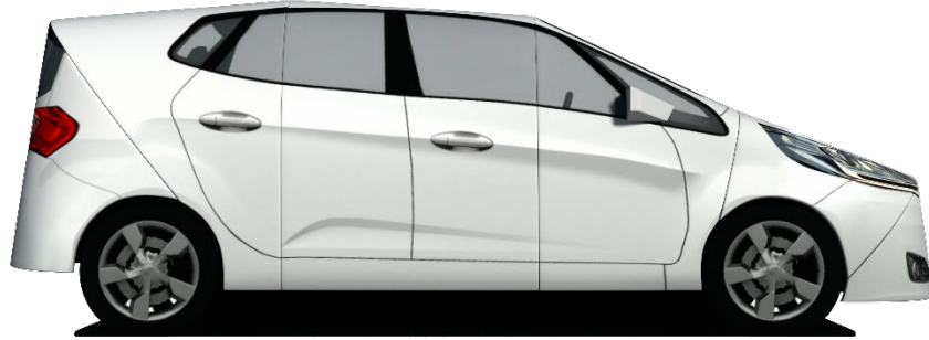
Figure 5-1: Global Vehicle Target (GVT)
