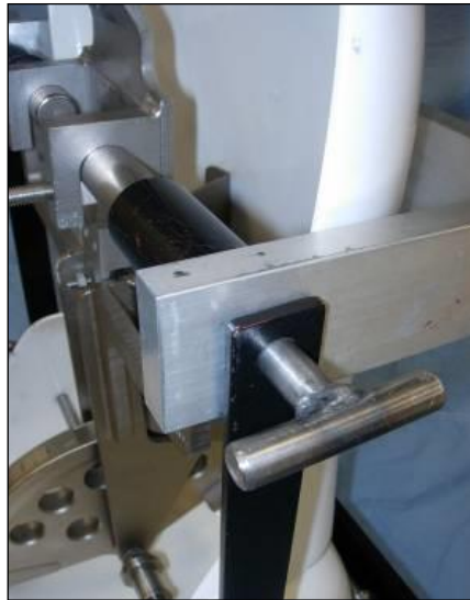
Figure 22: Weight hanger support pins inserted through weight hanger guide bars.
