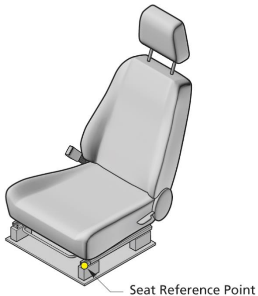
Figure 1: Definition of the Seat reference point.
