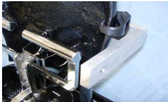
Figure 21: H-PM back pan held by retaining strap.
