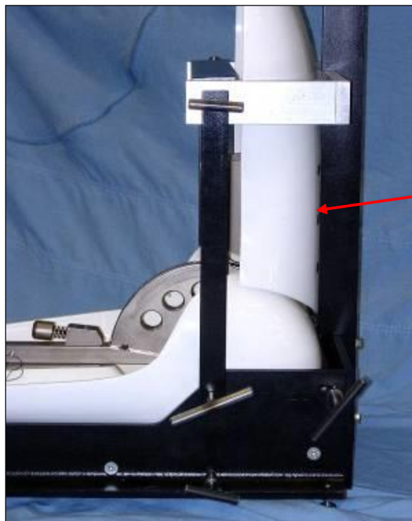
Figure 23: H-PM installed into the jig. A check should be made to ensure that the gap between the H-PM back pan and jig vertical support is no more than 4mm.
