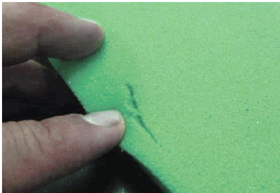
Figure 1 Small tears in rear surface of the foam
