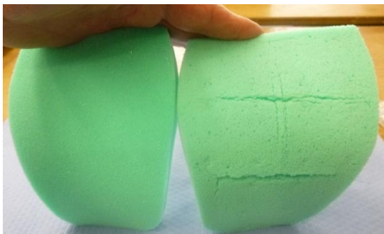
Figure 3 Face foam seen from back, new condition (left), replace if multiple large cracks appear (right)
