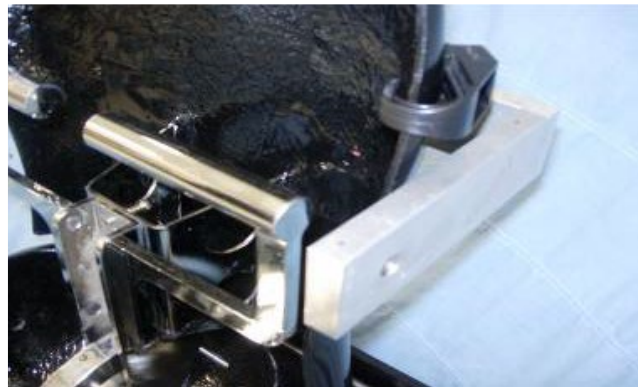
Figure 21: H-PM back pan held by retaining strap.
