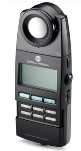
figure: Luxmeter Konika T-10A
