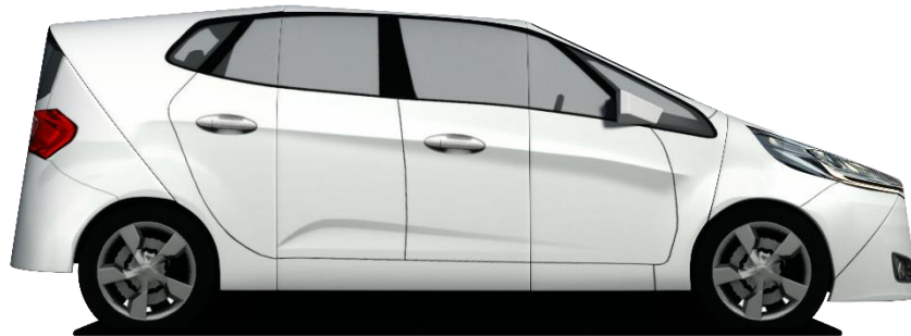
Figure 5-1: Global Vehicle Target (GVT)
