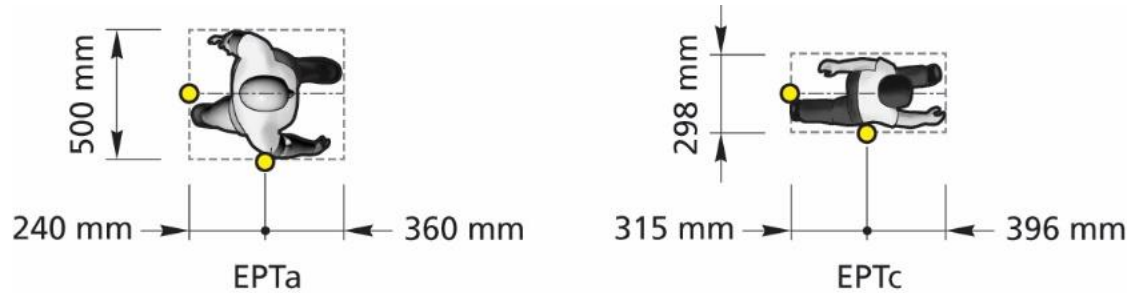
Figure 3-4: Virtual box dimensions around EPTa and EPTc
