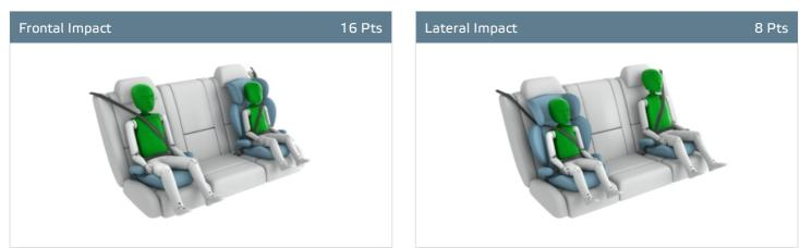
Restraint for 6 year old child: *Britax Römer Kidfix M i-Size OEM with Secure Guard* Restraint for 10 year old child: *Britax Römer Kidfix M i-Size OEM (CRS Seatback and Secure Guard removed*)
