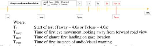
• The detection requirements for vehicle response vary depending on the response action of the vehicle and are listed alongside the vehicle response in 3.5.4.1. The detection requirement can be as low as gazes away of  $\geq 1$  second.
