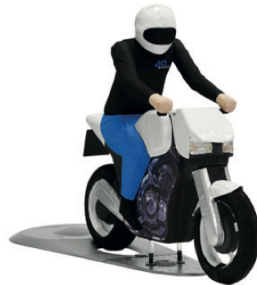
Figure 1. 4activeMC motorcycle target with the 4activeFB-small platform
