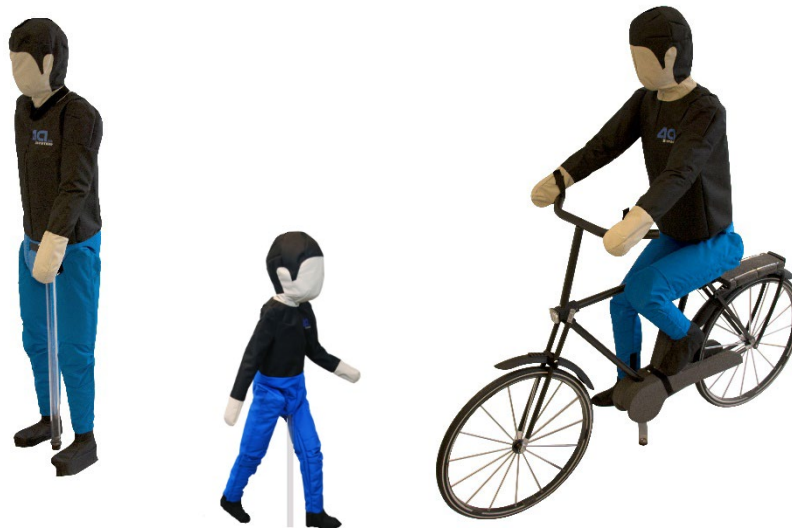
Figure 4-1 Euro NCAP Pedestrian Target (adult and child) and Bicyclist and bike Targets (EPTa, EPTc and EBT)
