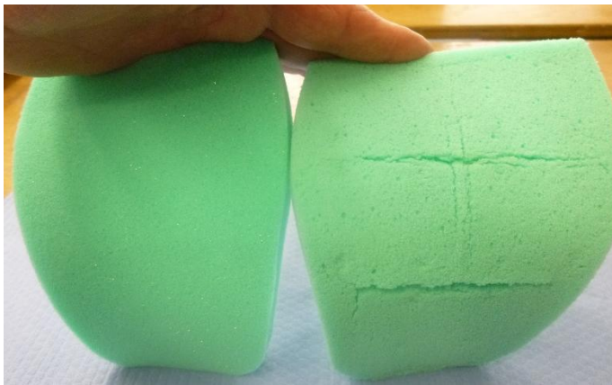
Figure 4 Face foam seen from the back, new condition (left), replace if multiple large cracks appear (right)
