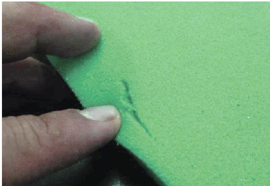
Figure 2 Small tears in rear surface of the foam
