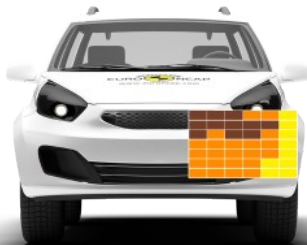
Mobile Progressive Deformable Barrier
